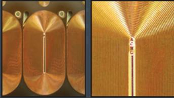
This complex copper micro-coil consists of four coils, each with 44 turns, layered one over another and series wound for a total of 176 turns per induction system and with an overall width of 2.3 mm (0.090") and length of 4.24 mm (0.167"). The conductor width is **12.5 microns** (0.0005") and the spaces between conductors are also **12.5 microns**. Conductor height is **7 microns** (0.0003"). A **10-micron** (0.0004") thick polyimide layer separates the four copper conductor layers.
