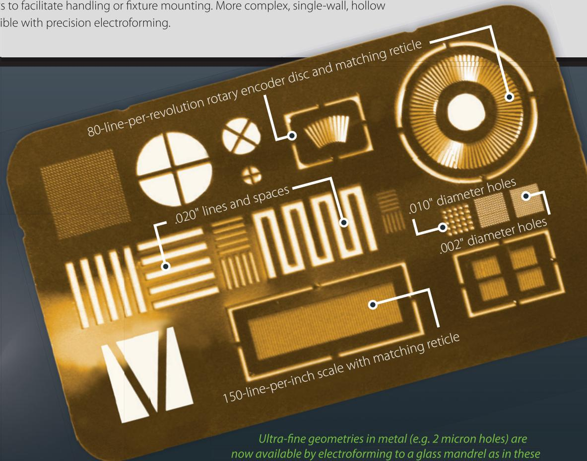
*Ultra-fine geometries in metal (e.g. 2 micron holes) are now available by electroforming to a glass mandrel as in these 40-microns-thick nickel cobalt samples over-plated with gold.*
