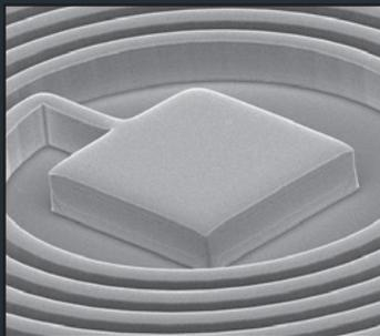
Metrigraphics' electroforming technology can fabricate high aspect ratio conductors (they are tall relative to their length and width). This electron microscope image shows a coil on a glass substrate. The width of the conductors is **10 microns** (0.0004"), and the height of the conductors is **25 microns** (0.001"). The spaces between the conductors are also **10 microns**. Dimensional tolerance is better than one micron.
